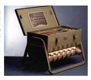
handling in addition to having multiple handles for moving by a 6 man crew. Input power to all units is 120/208 VAC three-phase. Outputs are protected by thermal-magnetic breakers, with ground-fault interrupters on single-phase output lines. All circuit breakers can be specified fungus-proof. Outputs are delivered by way of Class L circular connectors or NEMA wiring devices. The panels are finished in the various standard MIL-STD-595 service colors, including desert sand and camouflage.
